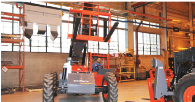
A VR642D telehandler is put through the paces after final assembly.
